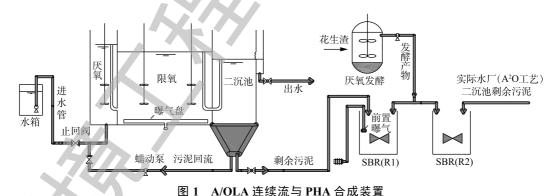
Fig. 1 Diagram of A/OLA continuous flow and PHA synthesis device
